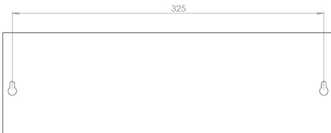
Drill and plug the wall with suitable plugs. Ensure that the screws will fit the back plate before drilling any holes. Ensure that the
